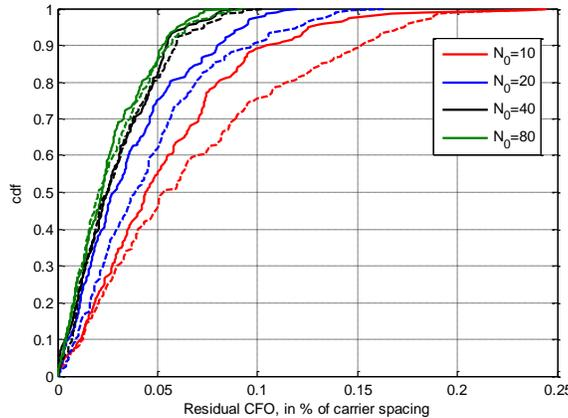
Figure 7 Residual CFO, in % of carrier spacing.  $\delta_{\Delta f} = 12.5\%$ ,  $d=160$  m. Solid lines:  $\tau=220$  samples, dashed lines:  $\tau=0$  sample.
