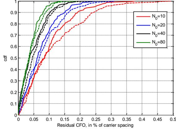
Figure 6 Residual CFO, in % of carrier spacing.  $\delta_{\Delta f} = 12.5\%$ ,  $d=250$  m. Solid lines:  $\tau=220$  samples, dashed lines:  $\tau=0$  sample.
