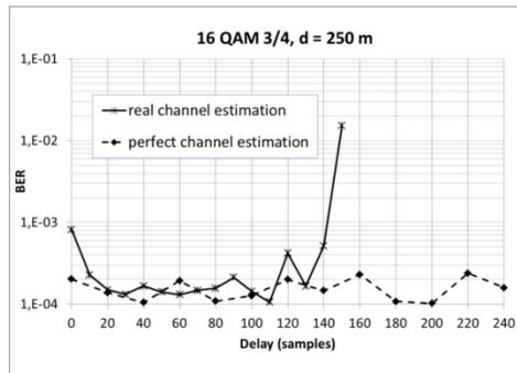
Figure 2 BER of CoMP FBMC with MRC at the receiver for different delays  $\tau$  between BSs.
