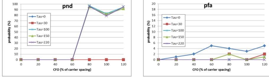
Figure 5 Estimation of the delay before CFO correction: probabilities of non detection and false alarm.  $d=250$  m.
