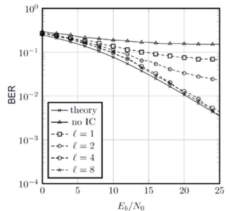
Fig. 3. BER performance of MF-SIC GFDM receiver considering different number of iterations (with parameters  $M=5$ ,  $K=128$ ,  $g[n]$  is a raised cosine pulse with roll-off of 0.4, 64-QAM and Rayleigh multipath channel with exponential decaying profile between 0 dB and -10 dB).
