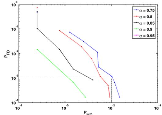
Fig. 6.  $P_{FD}$  over  $P_{MD}$  for the 5G “one-shot” random access with varying detection thresholds. The box illustrates the LTE feasible region.
