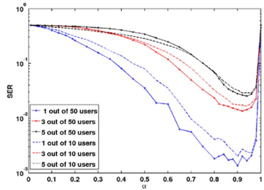
Fig. 5. Avg. BPSK SER in 5G “one-shot” random access (in 20MHz LTE-A setting) at SNR=20dB. Out of  $n=24576$  dimensions,  $m=839$  are used for CS.
